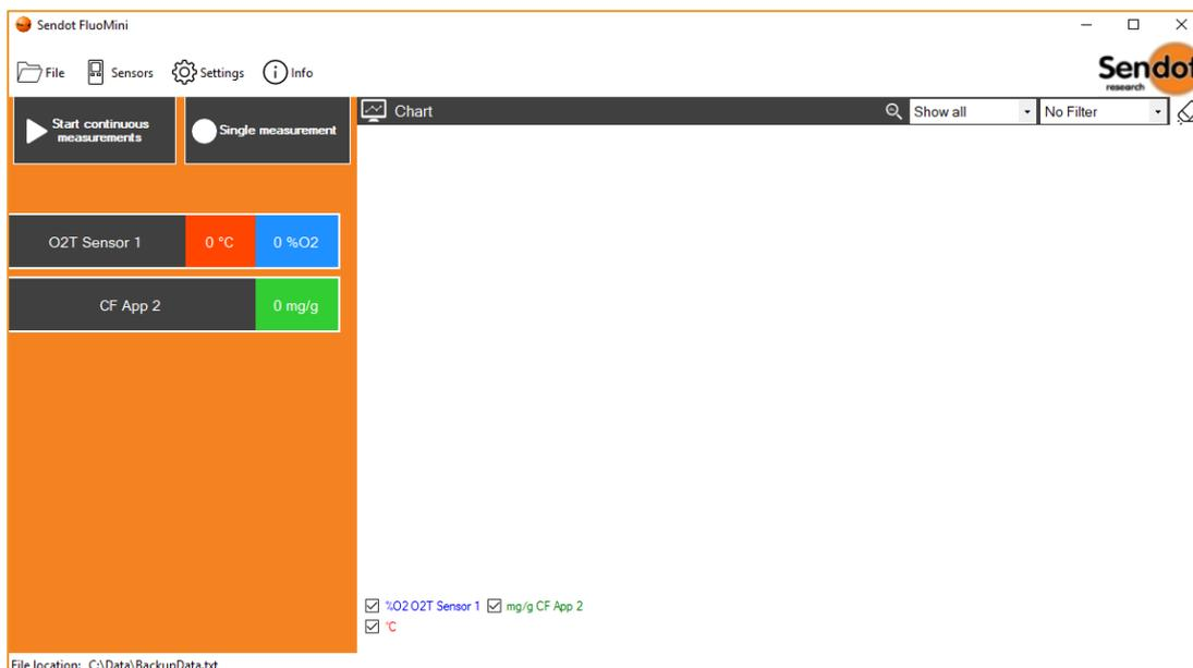
Once all ports have been checked, the FluoMini Software Suite will start and show all connected sensors on the left-hand side.
