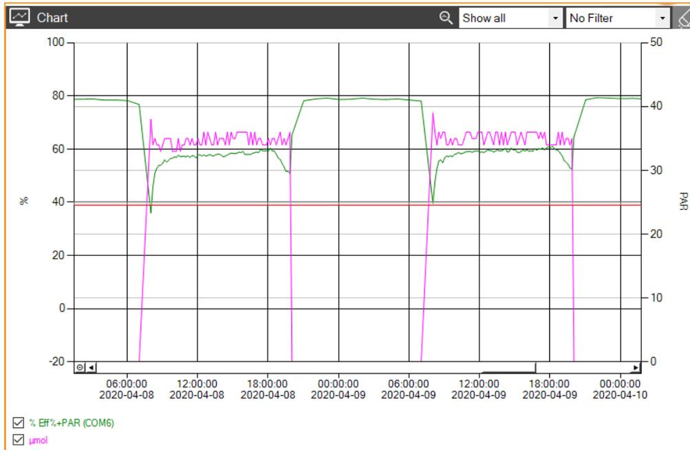
O<sub>2</sub>|T, CF and CF Seed you will only see one y-axis for the measurement value. In case of the Eff%+PAR sensor, two y-axis are visible – left-side for Eff% and right-side for PAR (see following picture).
