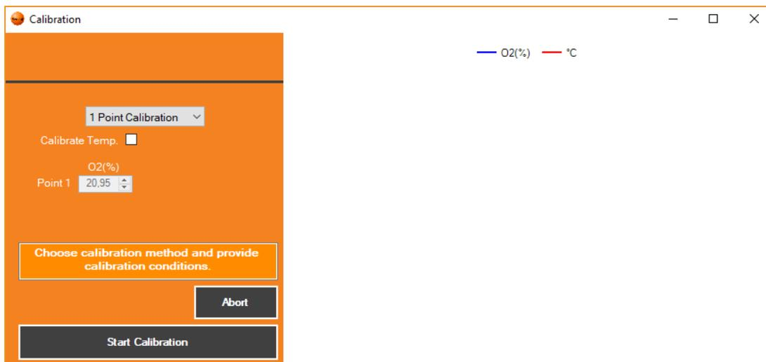
Here, you can calibrate each sensor. The software automatically recognizes the sensor type and shows the corresponding instruction to perform the calibration.
