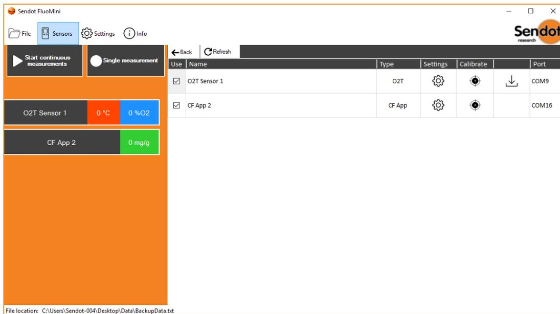
By selecting the checkbox to the left of the sensor name, you can choose to use the sensor when measuring. Only selected sensors will be visible in the graph.
