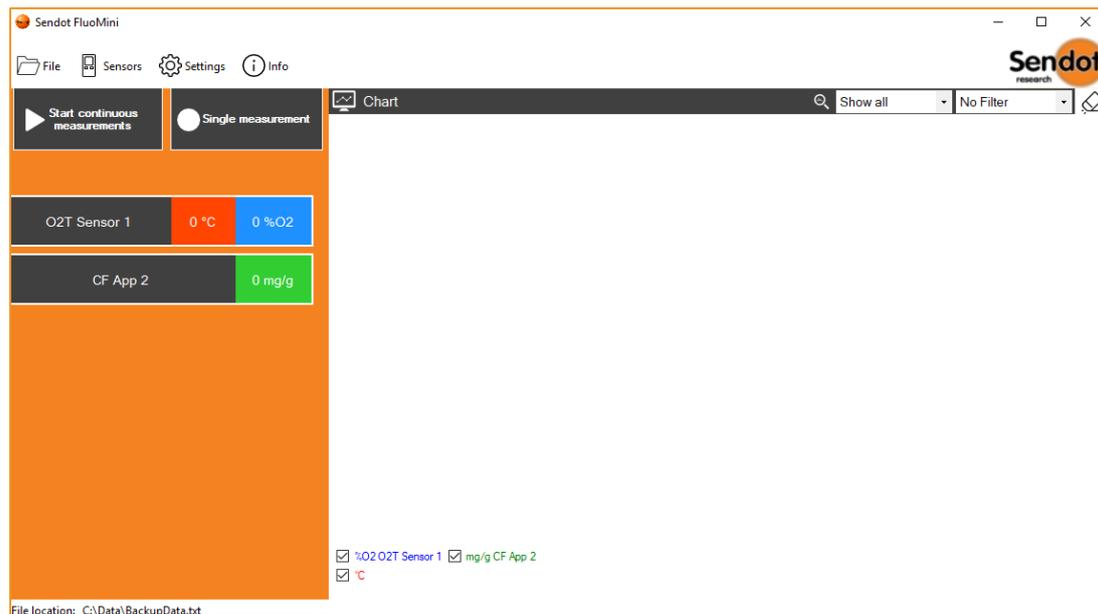
In the above example the main screen is shown. If no measurement has been performed or no data has been loaded, no chart is visible.
